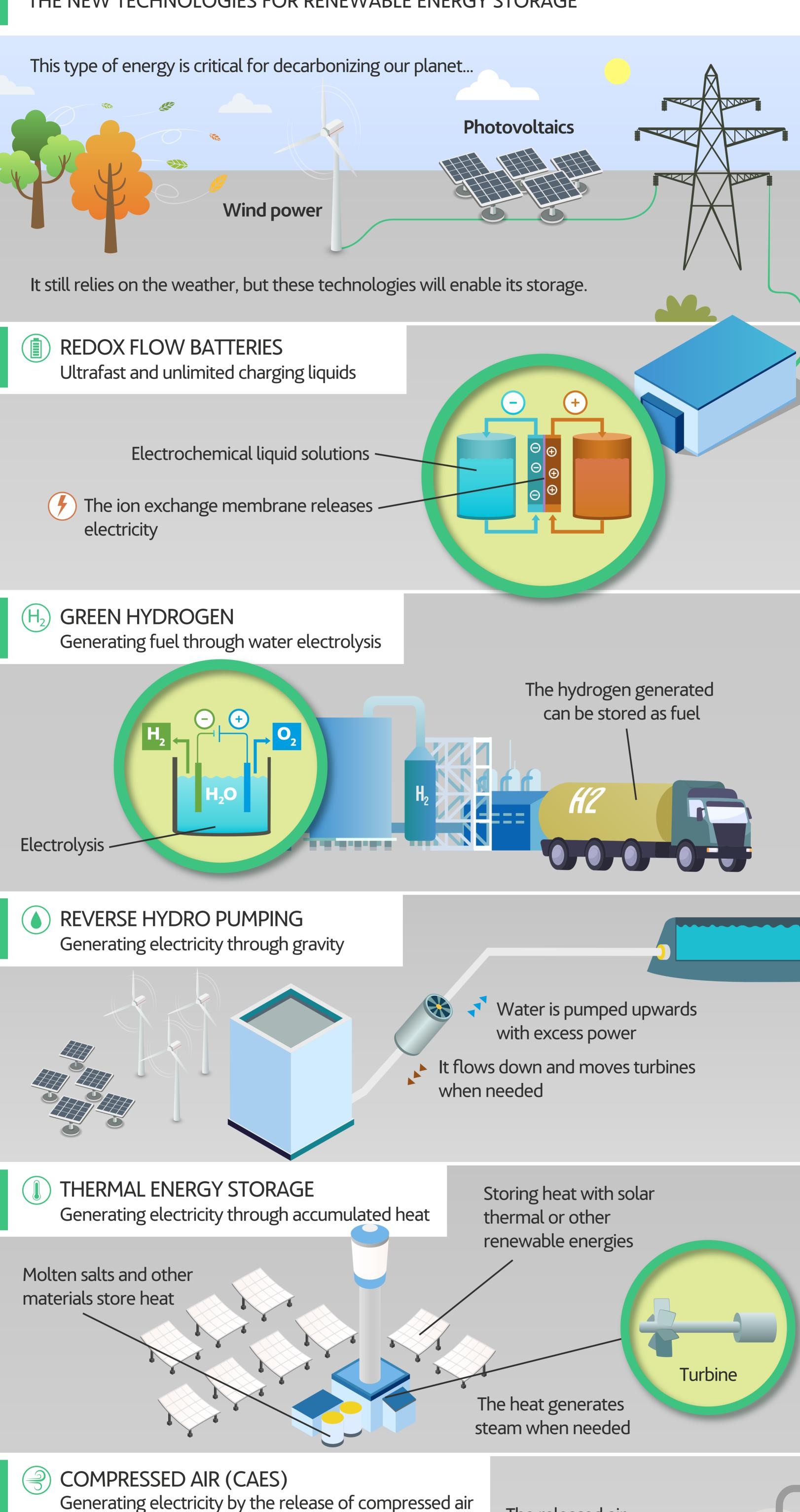
Air is compressed and pumped into underground cavities
